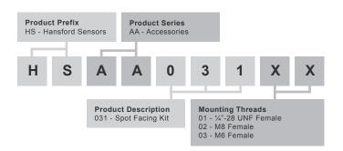
Spot Face Tool Only HS-AA001-1/4 - Ø32mm for 1/4"-28 UNF Thread HS-AA001-M6 - Ø32mm for M6 Thread HS-AA001-M8 - Ø32mm for M8 Thread
