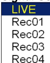
Every measurement can be taken from LIVE channels ( AC 1-4 or DC 1-4 ) or from RECORD ( see Recorder chapter for understanding). All records saved in the memory are displayed for selection. Select required item and press **OK** button. The selected signal source is also displayed in the Global window.
