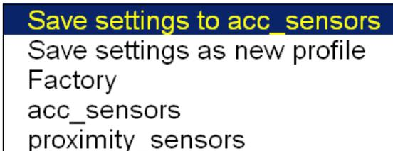
**Save settings to name** saves the parameters to the Profile, which was opened.
