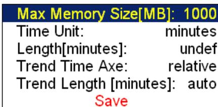
**Max Memory Size[MB]**      value            It enables partial savings of runup measurement. If the size of measured data exceeds the value, then data are saved and new runup is opened.
