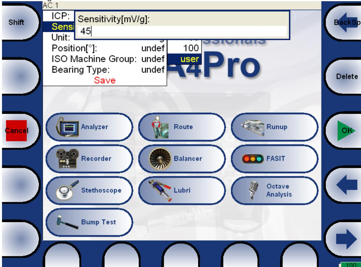
Now you can move the cursor, to use the **Delete** function. Press the **Shift** again and the buttons functions change back. When the value is correct, push **OK**. The menu with new value appears.
