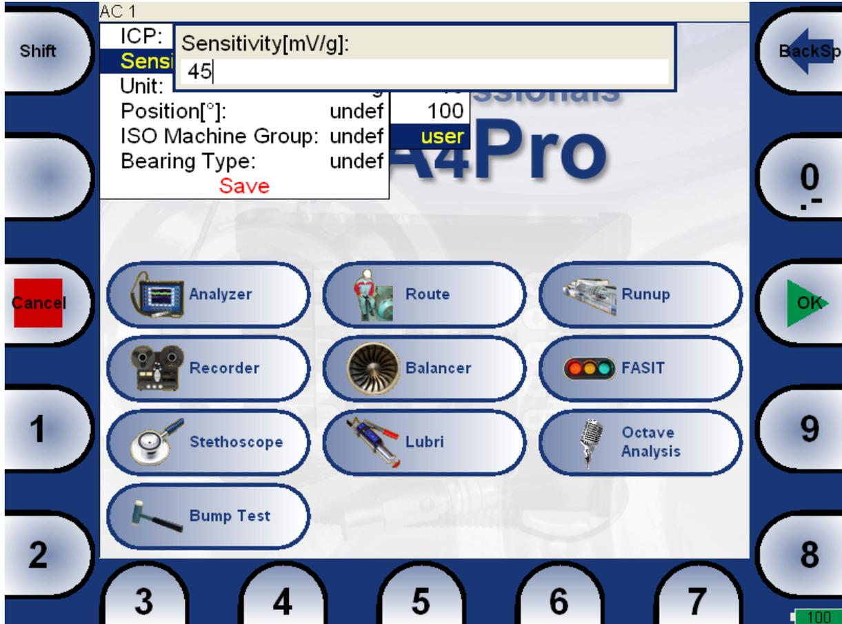
Use the buttons and enter required value (e.g.45). If you need to edit the value, push the **Shift** button. The buttons change the functions of buttons.
