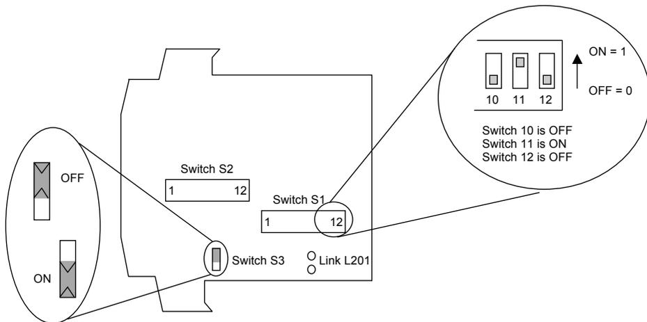
Switch S1, S2 and Link L201 configure the input type and range, and switch S3 configures the output type. Link L201 is connected only for potentiometer inputs which are not considered in this manual. The switch settings are explained in the next few pages. The diagrams refer to switch positions 0 and 1, with 0 being OFF and 1 being ON. This is illustrated in the picture above.
