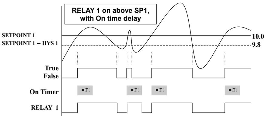
All 3 delays (or any combination) can be used at the same time if desired. Note that if the relay is tripped, both the 'on delay' timer and the 'on to off delay' timer can hold the relay in the tripped condition until both have expired (see picture below).
